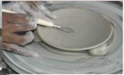
Trimming the saucer on the base and on the top of the saucer to finish the saucer
