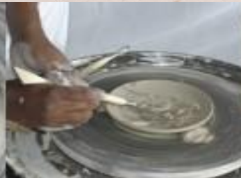
Trimming the saucer on the base and on the top of the saucer to finish the saucer
